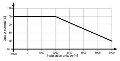
Figure 4-3 Mounting height derating
