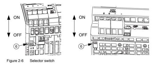
The two switches A and B are used to influence the output characteristic curve:
