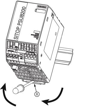
Figure 3-1 Mounting/removal (example 6EP3436-8SB00-0AY0)
