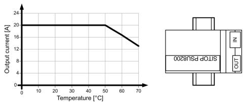
Figure 4-4 6EP3436-8SB00-0AY0 mounting position (1)
