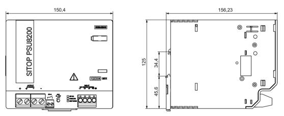
Figure 2-9 Dimension drawing 6EP1437-3BA10
