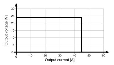
Figure 6-4 6EP1437-3BA10 single operation output characteristic curve
