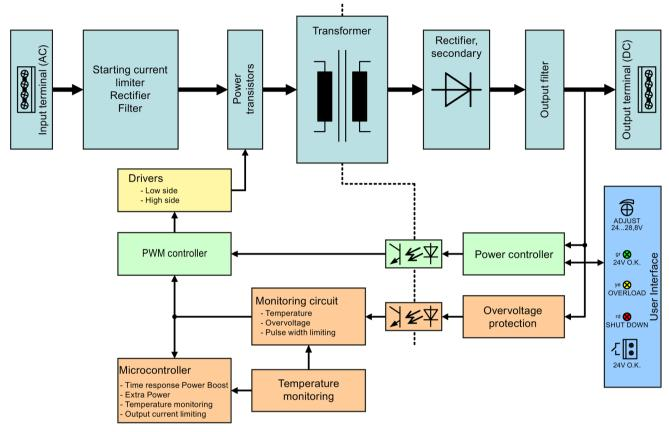
Figure 2-7 Block diagram
