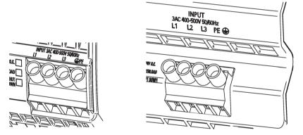
Figure 5-1 Line supply connection
