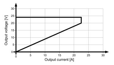
Figure 6-7 Output characteristic curve 6EP3436-8SB00-0AY0 latching shutdown
