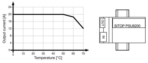
Figure 4-5 6EP3436-8SB00-0AY0 mounting position (2)
