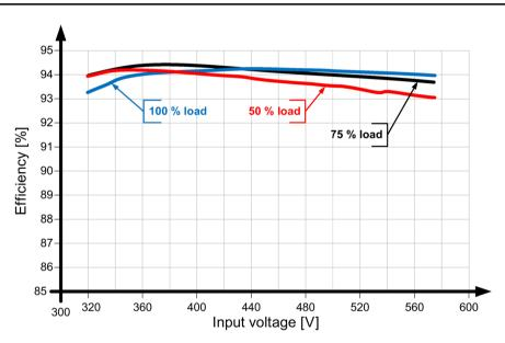
Figure 6-9 Efficiency 6EP3436-8SB00-0AY0
