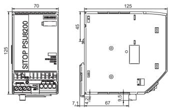
Figure 2-8 Dimension drawing 6EP3436-8SB00-0AY0
