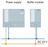
Figure 9-6 Buffering brief power failures using the SITOP PSE201U buffer module
