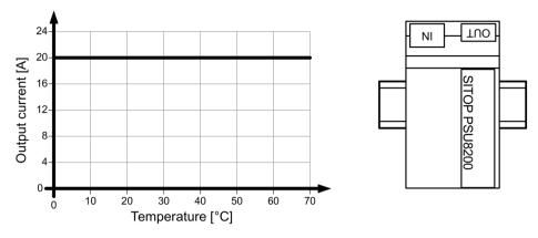
Figure 4-6 6EP3436-8SB00-0AY0 mounting position (3)
