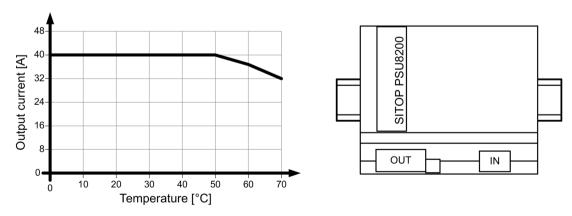
Figure 4-2 6EP1437-3BA10: Output current in the standard mounting position
