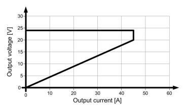
Figure 6-8 6EP1437-3BA10 latching shutdown output characteristic curve
