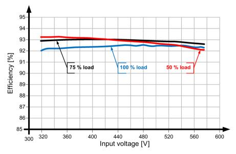
Figure 6-10 Efficiency 6EP1437-3BA10
