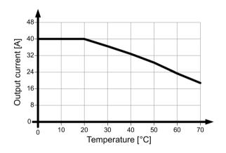
Figure 4-10 6EP1437-3BA10 mounting position (2)
