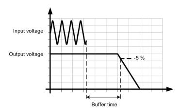
Figure 6-1 Power failure buffering
