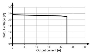
Figure 6-5 Output characteristic curve 6EP3436-8SB00-0AY0 parallel operation
