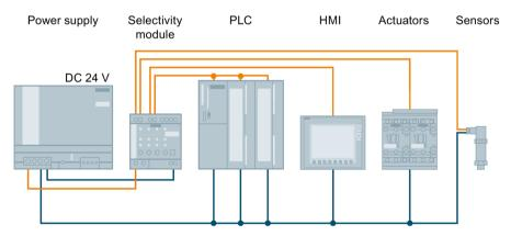
Figure 9-5 Electronic protection of 24 V consumers with the SITOP PSE200U selectivity module
