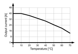
Figure 4-9 6EP1437-3BA10 mounting position (1)
