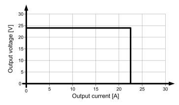
Figure 6-3 Output characteristic curve 6EP3436-8SB00-0AY0 single operation
