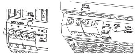
Figure 5-2 Output connection
